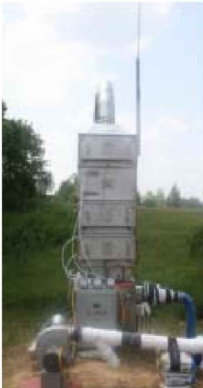
Front and side view of the igloo filtration system (IFS) proposed for use at Blue Grass Chemical Activity.
